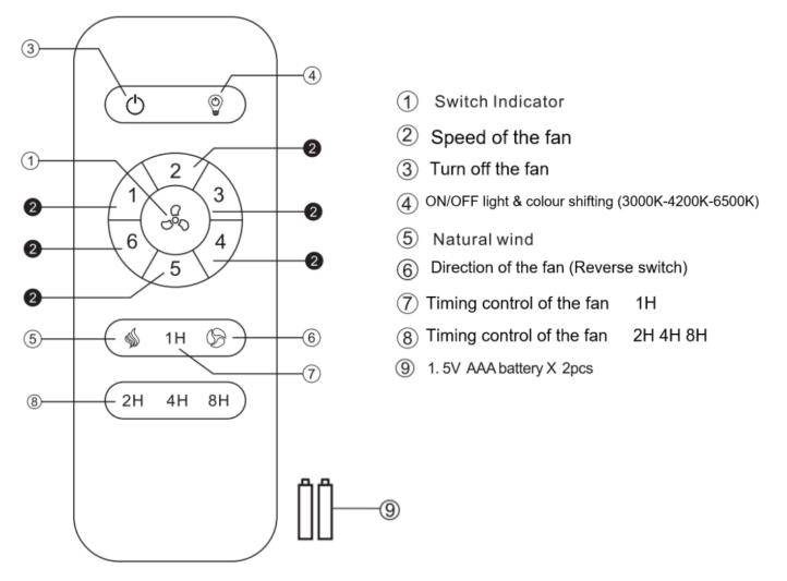
The remote has memory function. If the fan or light is turned off by the isolating switch over 7 seconds, the next time to turn on the fan or light will be on last setting.
