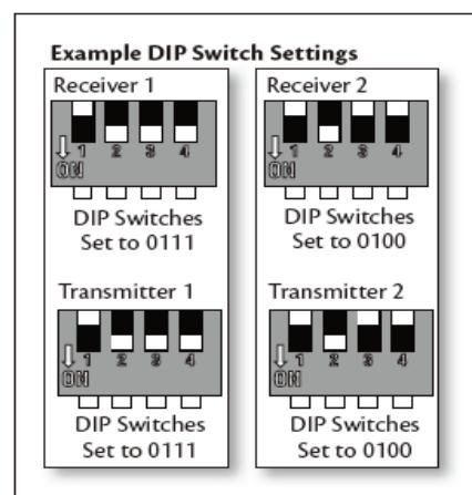
**Fig. 10 Interruptor DIP del receptor**
